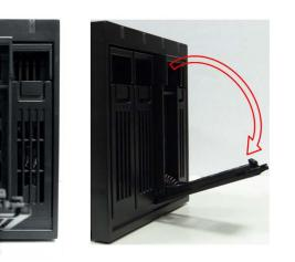
Hard Drive Installation Installing a 3.5" HDD
